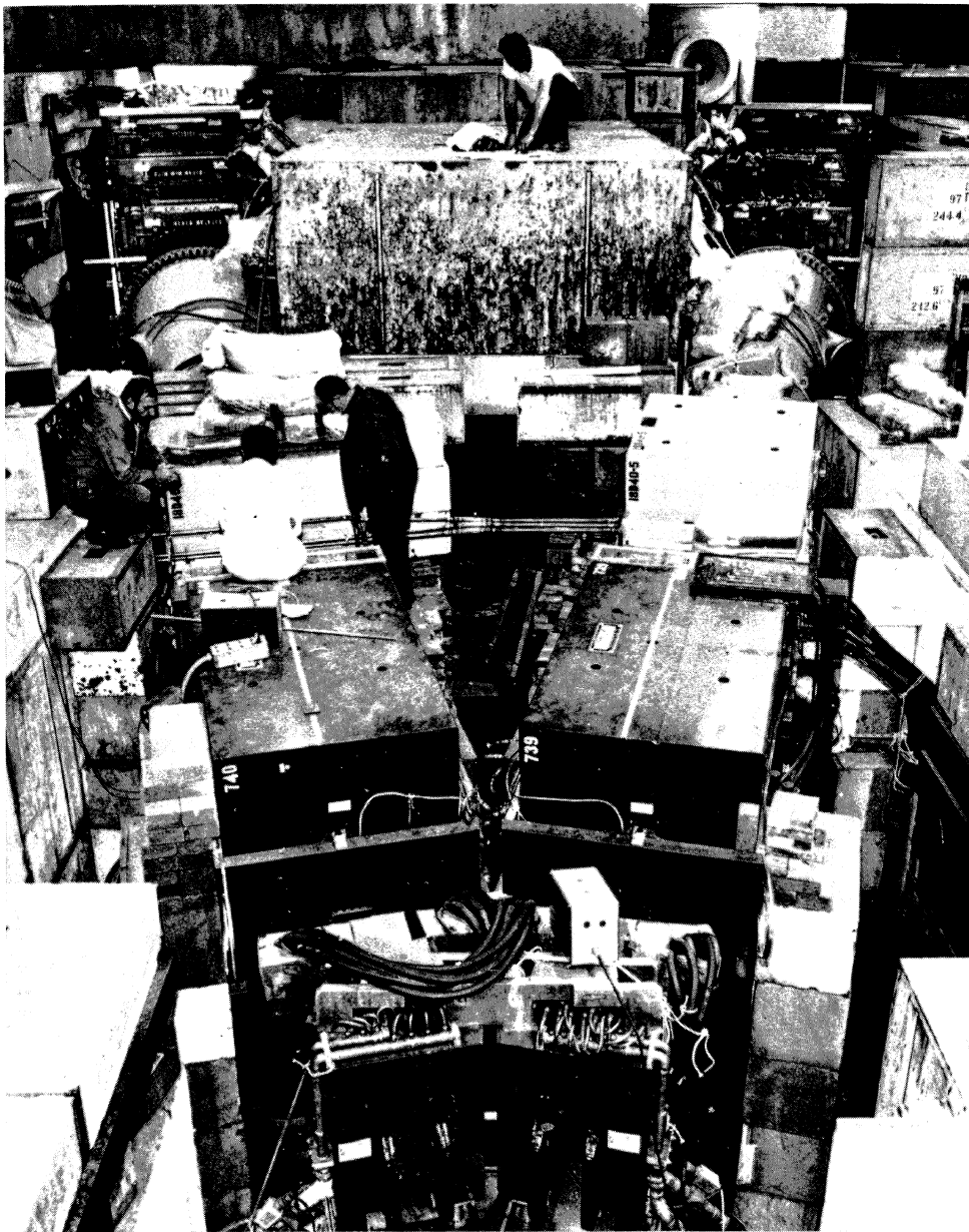
The detection system of the experiment at Brookhaven which spotted the new particle. It consists of two symmetrical spectrometer arms, 20 m long. In the foreground in each arm are three magnets. They are followed by Cherenkov counters (looking like cement mixers) to identify particles (in addition to Cherenkovs in the magnets) and, finally, multiwire proportional chambers which determine precise particle positions. (Photo Brookhaven)
